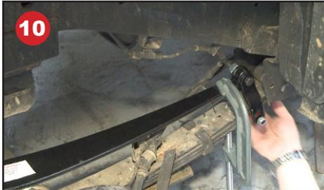
Hold down (or G Clamp) one side of the Superspring and place the bolt, sleeve and bush back onto the shackle under the vehicle leaf spring using the recommended shackle holes. Tighten the lower shackle bolt only.
