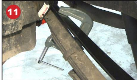
Using the 'G' clamp, pull the other side of the Superspring into position.
